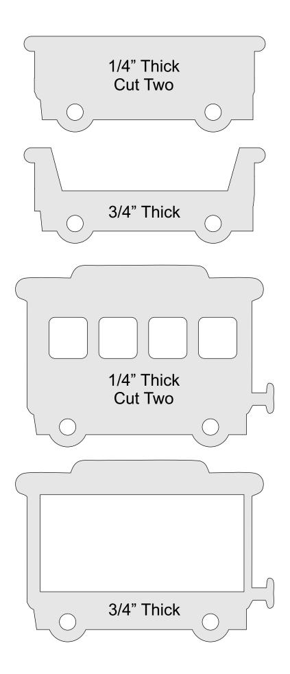
1/4" diameter holes in the wheels. Cut the axles from 1/4" wooden dowel rod.
