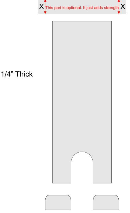
Test the position of these stops for the thickness of you smart phone
