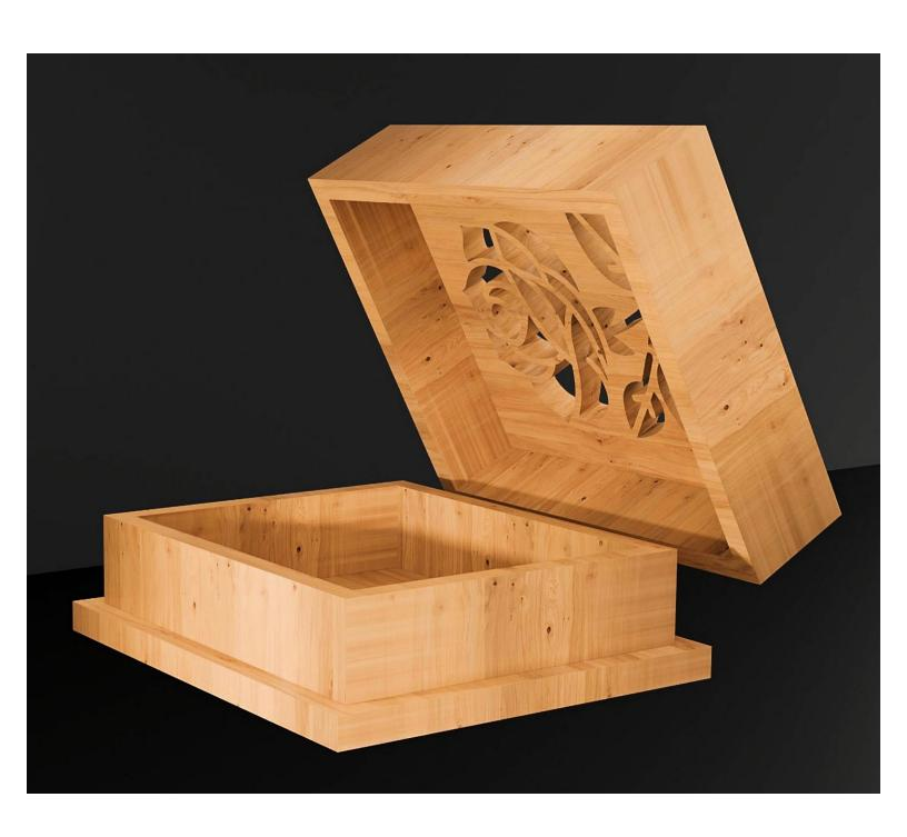
Do not use a blade smaller than a #5 to cut the segmented box interior cut line. You will need to make precise corner cuts so a larger blade may be too be difficult to turn. You need the drilled hole to be straight so consider using a drill press if you have one. One other option is to drill at each corner so you have room to turn the blade easily
