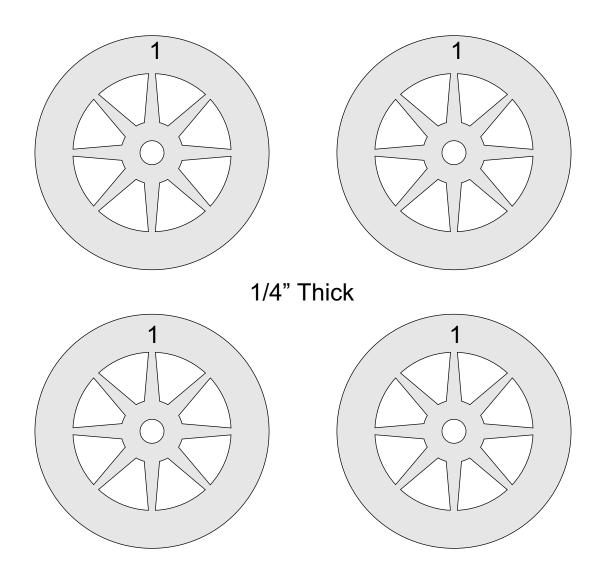
Drill 1/4" diameter holes for the axles.
