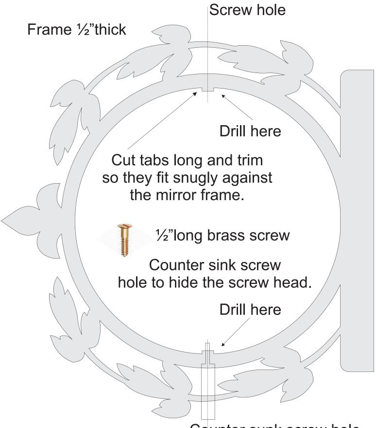
Counter sunk screw hole Drill holes for screw before cutting pattern.
